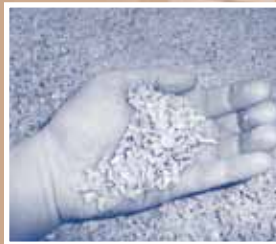
Plastic cartridges are ground down to be recycled into new products.
